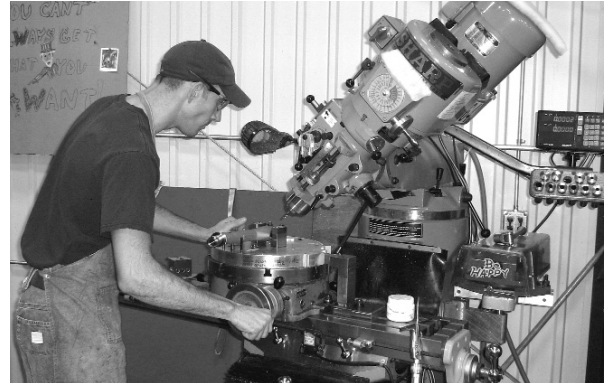
Sterling Machine's new scholarship intern, Jason Cebula, performs a manual operation for spot facing and drilling a hole in a gun mount detail for a Black Hawk helicopter. He works with a mentor in Sterling's toolroom and will learn various manufacturing processes, including manual machining, CNC machining, assembly, production control, shipping, inspection and engineering.
